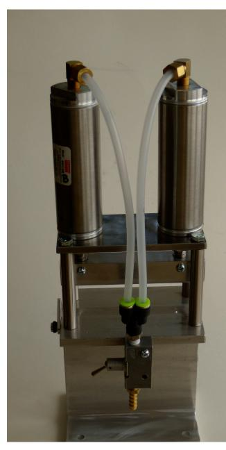
When the toggle clamp is flipped the upper V block will come down with considerable force. **Be sure to keep your fingers out of the way!** It is best to just move the toggle switch slowly which will bleed air into the cylinders and cause the upper V block to descend slowly onto the shaft.
