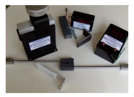
floating V block which is placed on the top of the shaft. An upper U shaped bracket contains a slip clutch which applies the force to clamp the shaft between the two V blocks. When tightened, the clutch will slip with about 300 pounds of force on the shaft. To provide accurate readings the Clamping unit must be firmly mounted to a work bench and the bench itself must be reasonably solid. A loose clamp or wobbling of the bench will lower the frequency by one or two
