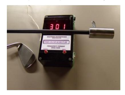
alignment is a bit below the sensors. The grip will result in dampening and lower the frequency by about 5 to 7 cpm.
